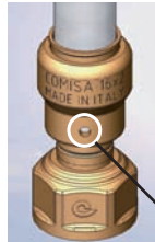
4. Push the multilayer pipe into the fitting, up to the pipe stop by checking the correct insertion depth through the inspection window designated for the visual control of the position of the pipe
