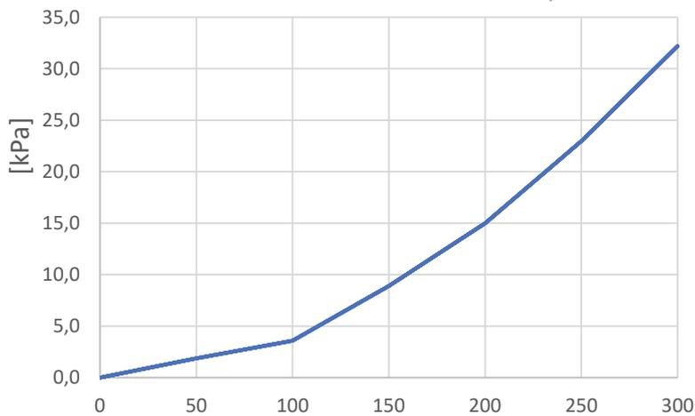
Pressure drop chart for water at temperature 15°C
